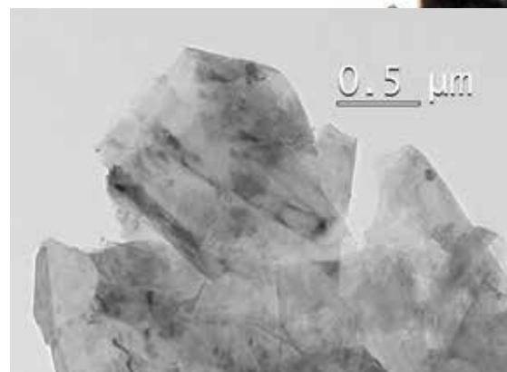
Electron micrograph (TEM) shows various few-layer thick flakes with thicknesses mainly ranging from 6 to 10 layers.
